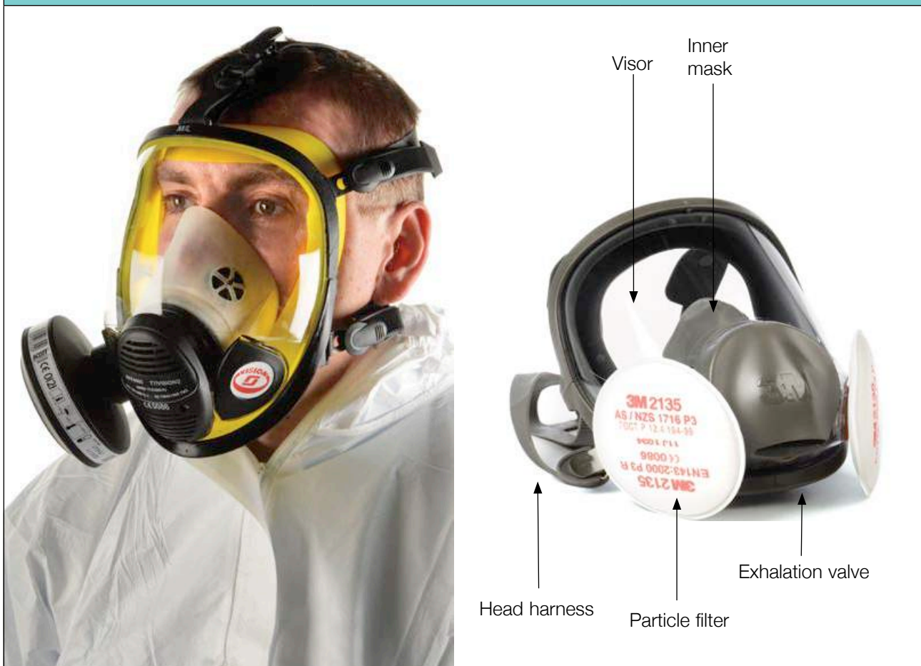
Figure 11 Full face mask respirators – particle filter
