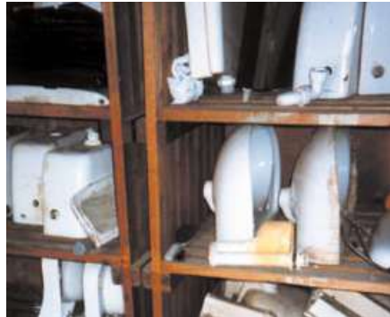
Figure 40 Asbestos-reinforced toilet cistern
