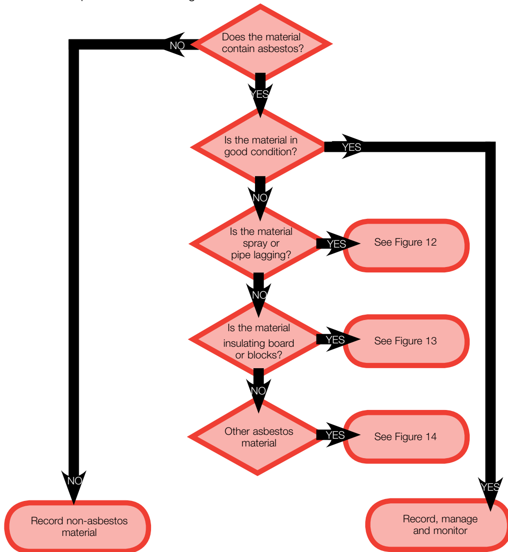
Figure 11 Materials suspected of containing asbestos
